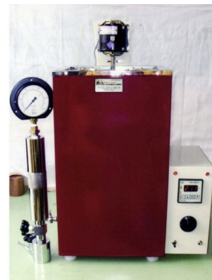
REID VAPOUR PRESSURE
